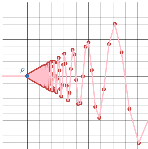
Figure 4.4: An illustration of g in the case that E = 0 \cup \{1/n \mid n \in \mathbb{N}\} and f(x) := \lim_{z \rightarrow x^-} \frac{\sin(x)}{x} (Desmos).
